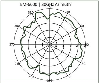
Radiation Patterns scaled at 3dBi/Div. Azimuth measured at 0deg offset from electrical center of the antenna.
