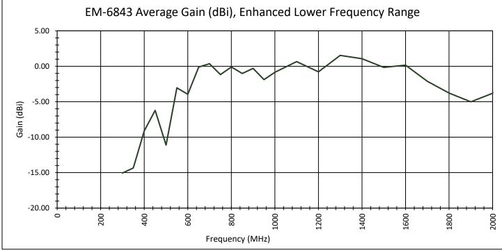
\*Maximum Gain determined from scans at all radiation angles and elevations. Data shown is typical, not guaranteed.
