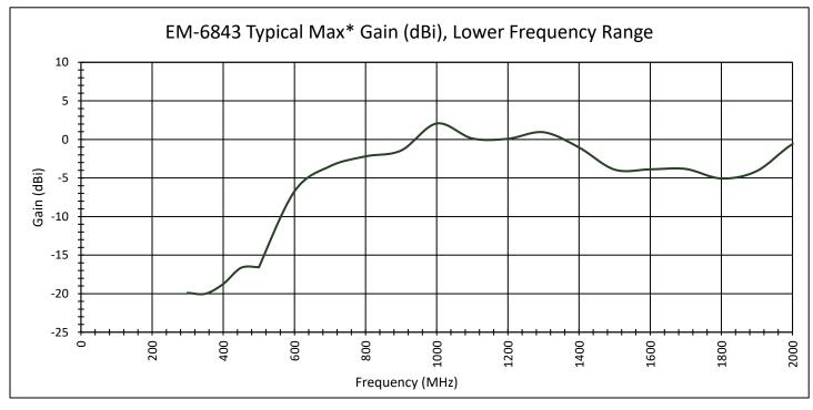
\*Maximum Gain determined from scans of Azimuth axis at 0 deg Elevation. Data shown is typical, not guaranteed.
