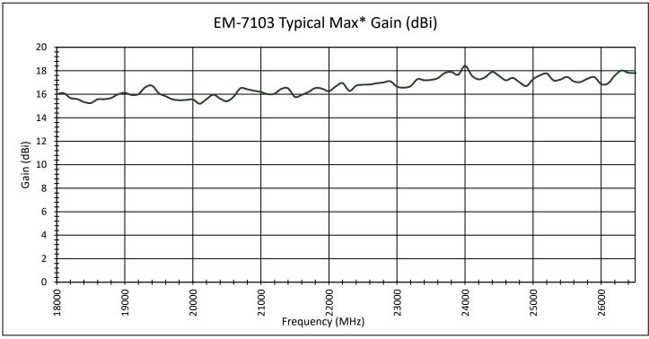
\*Maximum Gain determined from scans at all radiation angles and elevations. Data shown is typical, not guaranteed.
