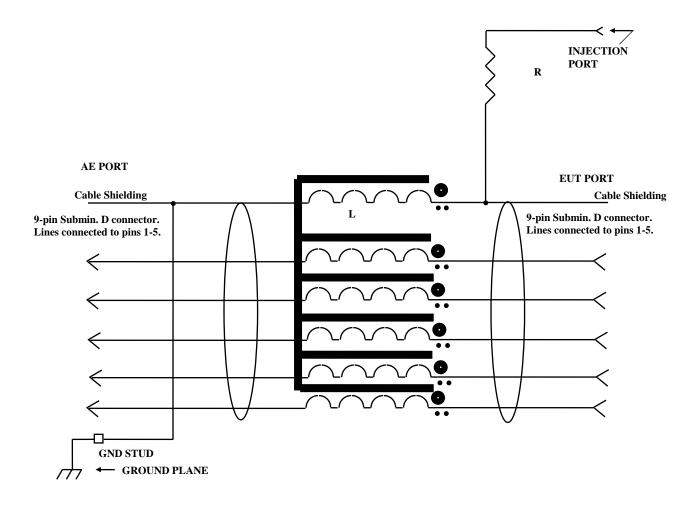
NOTE:  $R = 100 \ \Omega, \ L \geq 280 \ \mu H$  Ferrite Beads - as required.
