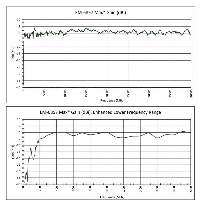
\*Maximum Gain determined from scans at all radiation angles and elevations. Data shown is typical, not guaranteed.
