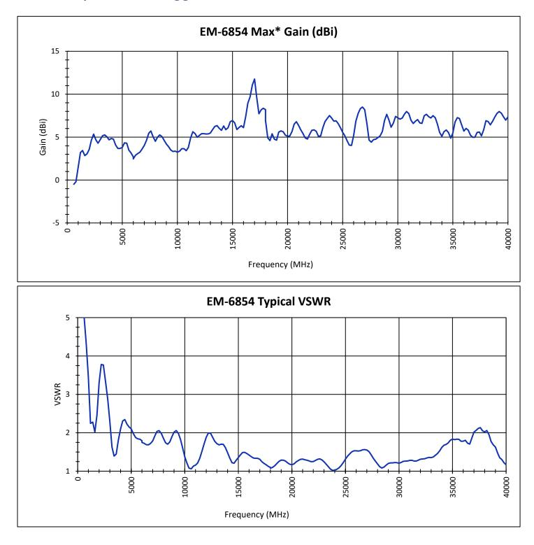
\*Maximum Gain determined from scans at all radiation angles and elevations. Data shown is typical, not guaranteed. Specifications subject to change without notice, unless otherwise specified. Product is manufactured in Johnstown, NY, U.S.A.
